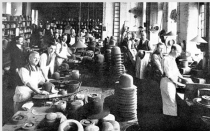
A picture taken inside Hall and Phillips, showing the production of felt hats. Many thanks to Peter Lee (nuneatonhistory.com).
